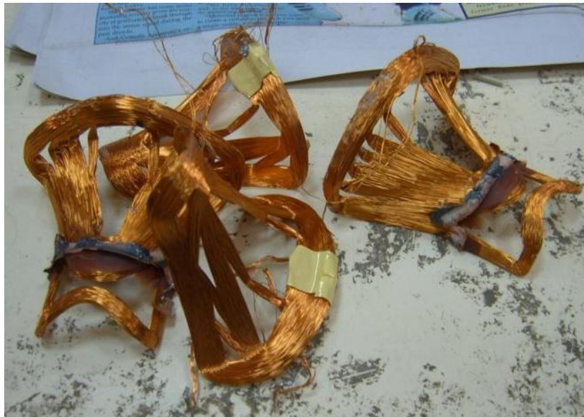
Photo 7 Pure copper retrieved from the yokes of CRTs
